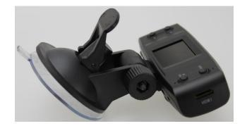
The suction cup should have a protective plastic disk that you will have to remove before it will work.
