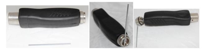
Your GS3000 should have come with a thin metal rod, which is designed to inset into the hole at the end cap of the GS3000. The rod should give you a handle to pull/push on to unscrew the end cap. Be careful, because some models have a spring under the end cap, so it may fly off once it is completely unscrewed.
