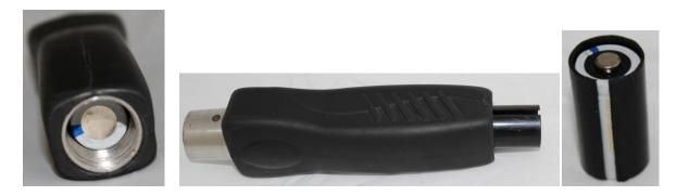
Now that both the end cap and the inside screw are removed, you should be able to see the negative side of the battery to the GS3000. Turn the device upside down over your hand and shake a little. The battery should fall out of the GS3000. The battery should be surrounded by a plastic tube. If it is not, check inside the GS3000 to see if it got stuck. If it is stuck, there should be enough room to stick your finger inside and pull it out.
