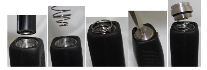
The unit should now be grounded, simply put the new battery inside the plastic tube, and put both back inside the unit (positive side of the battery face down). Place the battery spring (the smaller end goes in first) and screw the inside screw back in place. Replace the end cap (use the metal rod to help) and you will have successfully grounded and replaced the battery of the GS3000.
