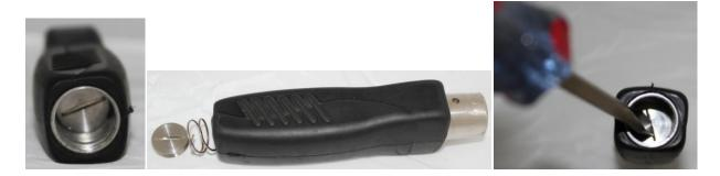
Once the end cap is removed you should be able to see inside the GS3000, and you should see a metal disk with a straight dent in it. This is just a large screw, and should be unscrewed with a flat head screw driver. This screw also has a spring underneath, so be careful of the screw flying out.
